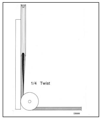
Figure 23. Drive Pulley to Idler Adjustment
